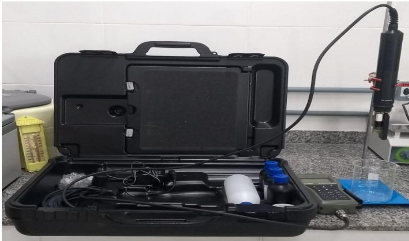
Sonda Multiparâmetros Hanna Instruments HI 9829
